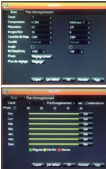
**Base [Basic] tab:** Allows you to choose the size, compression, frame rate (No. of images per second), sound recording/no sound recording (if an audio source is connected to RCA (phono) inputs 1 to 4 - option not available for the other channels).
