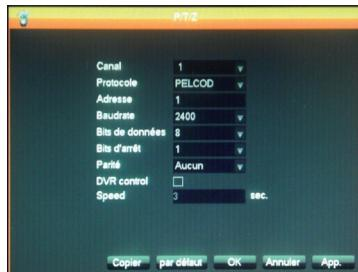
Used for configuring the wired output settings for controlling motorised PTZ cameras (not included). To be used in conjunction with the **P/T/Z** menu above and the motorised camera setup (for further details, please refer to the motorised camera user manual).
