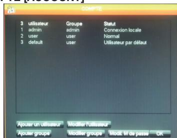
This displays the IDs and passwords used for logging in to the monitor (including the default admin account/password). This section is used to create additional users should you not wish to divulge the default "admin" account and password. It also allows you to change existing accounts and passwords.
