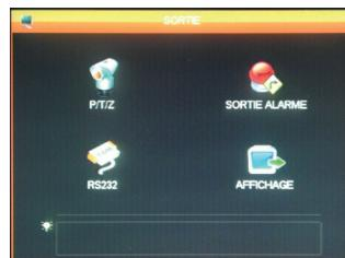
This menu is used to manage and control motorised cameras, the display of visual alerts and other display functions.
